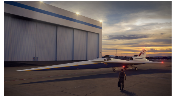
Figure 2. The X-59's unique design reduces the sonic boom to a quieter sonic thump.
