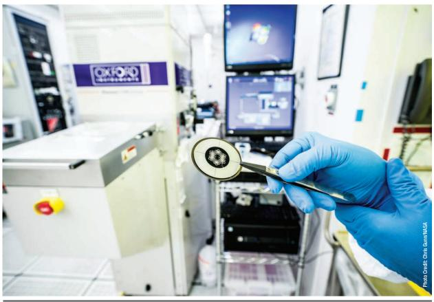
More than a work of art, the etched black silicon pupil masks are designed to absorb straylight in coronagraphs.
