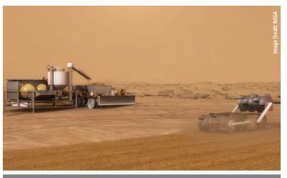
This is an ISRU system concept for autonomous extraction of water from the Martian soil.
