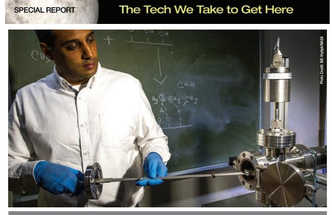
Goddard engineer Vivek Dwivedi won a flight opportunity to show that an advanced thin-film manufacturing technique called atomic layer deposition, or ALD, could apply wavelength-specific reflective coatings on a sample — the first time ALD will be tried in space.
