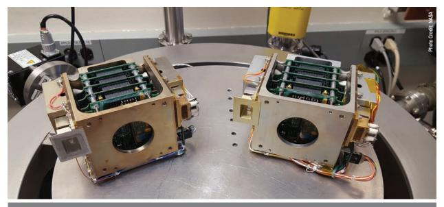
The lon-Neutral Mass Spectrometer, an instrument created by Nikolaos Paschalidis, and flight spare are shown here before they were delivered in preparation for the Dellingr launch.
