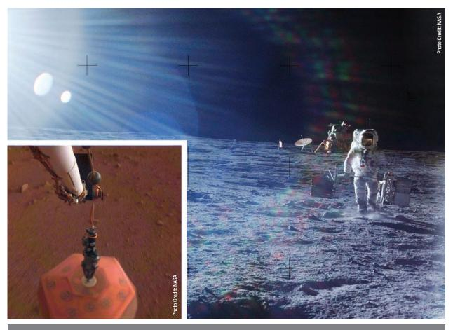
A next-generation seismometer could be deployed autonomously, unlike the systems shown here. Main photo. Apollo 12 astronaut Alan Bean carries the Apollo Lunar Surface Experiments Package to its deployment site on the Moon. The inset image on the left shows the deployment arm placing MarsInsight's seismometer system.
