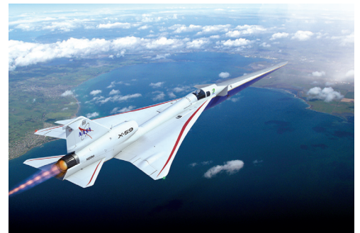
Figure 2. The X-59 is designed to fly supersonically without creating a sonic boom.
