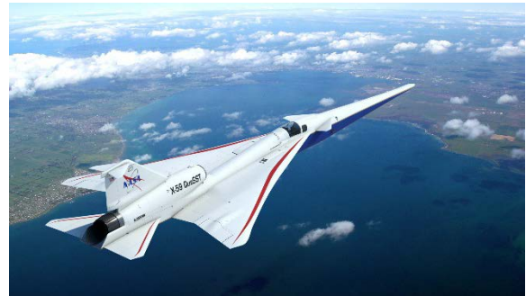
Figure 2. The X-59 is designed to fly supersonically without creating a sonic boom.
