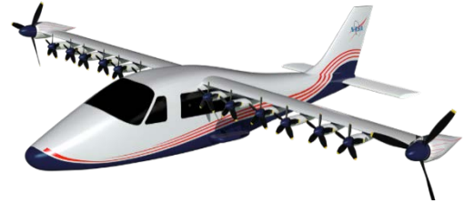
Figure 1. The X-57 is powered by electricity.
