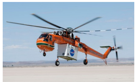
Figure 7. This S-64 heavy-lift helicopter uses the tail rotor to balance out the torque created by the rotor. Credit: NASA, Tony Landis
