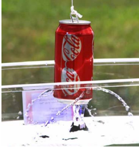
Figure 3. The water coming out of the holes causes the can to move
