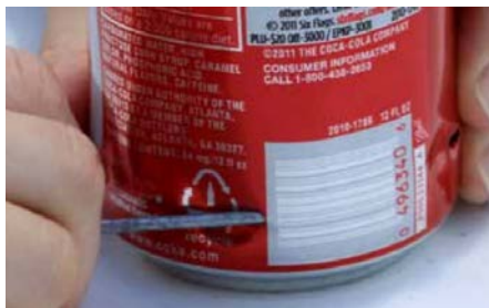
Figure 2. Use the nail to make holes near the bottom of the can
