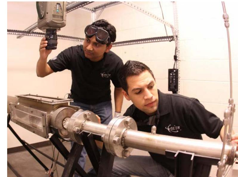
Research assistants in the Center for Space Exploration Technology Research set up a laboratory-scale turbine combustion rig and high-speed camera. Image Credit: University of Texas at El Paso, cSETR University Research Center
