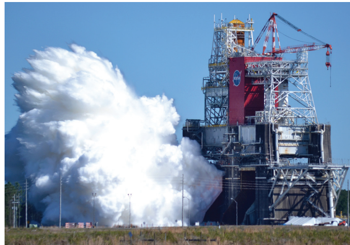
Artemis I core stage green run test in the B-2 test stand at NASA's Stennis Space Center.
