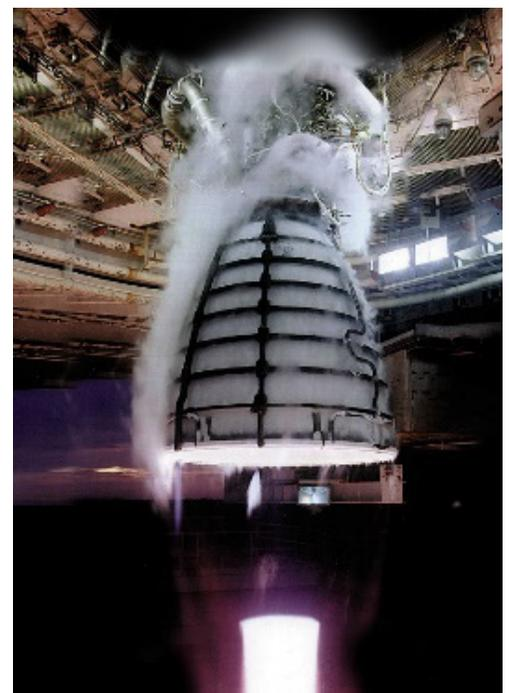
RS-25 engine undergoing a hot-fire test. (NASA)
