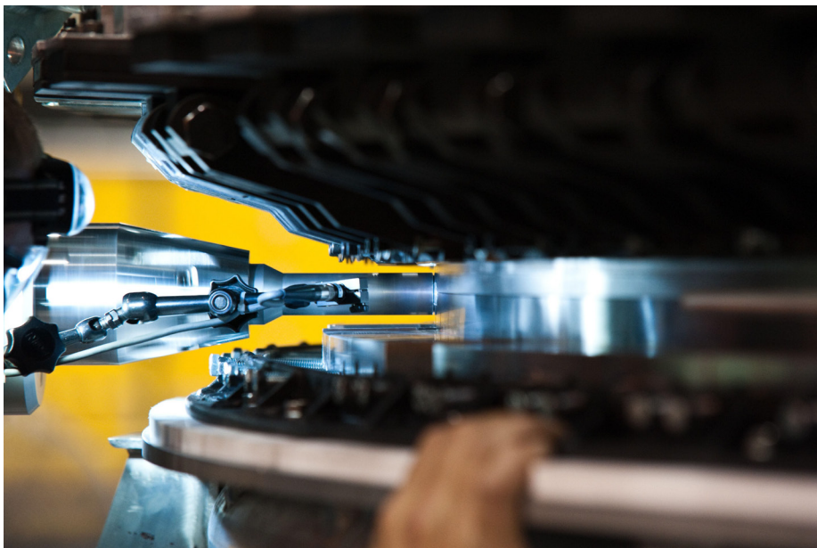
Orion's bulkhead and nose cone are joined using friction stir welding at NASA's Michoud Assembly Facility. (NASA)
