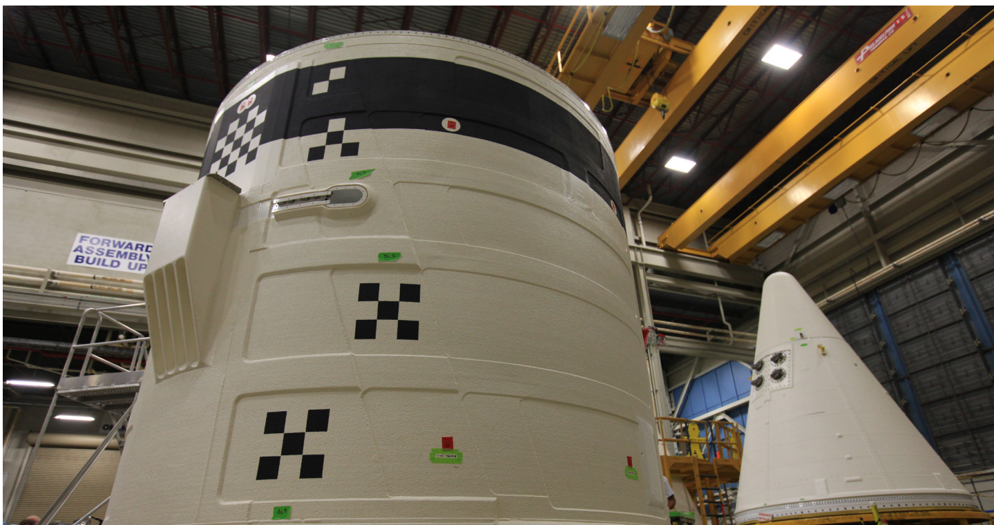
The forward skirt assembly includes the nose cap and the forward skirt, or top part, of the SLS rocket booster
