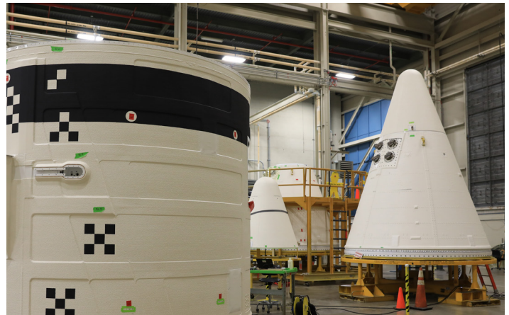
Booster frustum (front) and nose cap (back) for Artemis I
