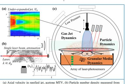
(a) Axial velocity in rarefied jet, acetone MTV, (b) Particle number density measured light attenuation, (c) Schematic of facility for PSI experiments.
