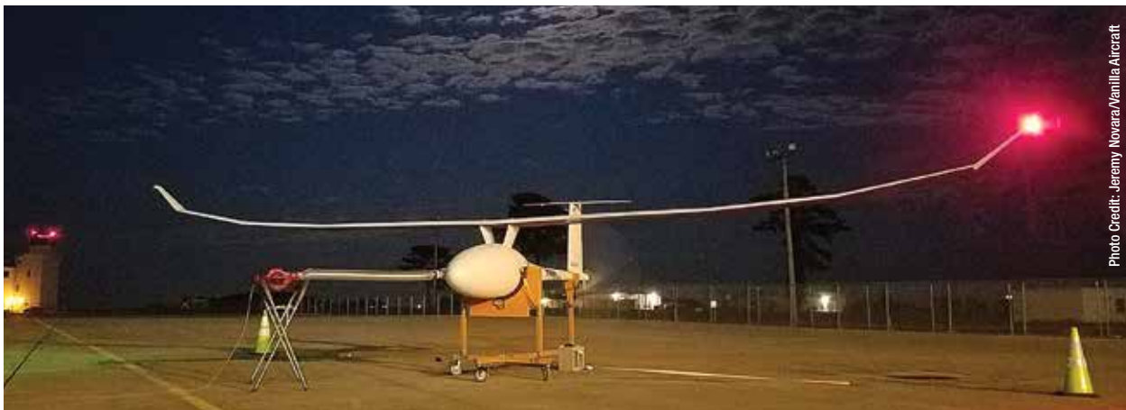
The VA001 can carry 35 pounds of payload, flying at 500 to 15,000 feet above sea level. Its primary attraction — and the primary reason NASA funded its development through the SBIR program — is its ability to carry out research over some of the most forbidding locations on Earth.
