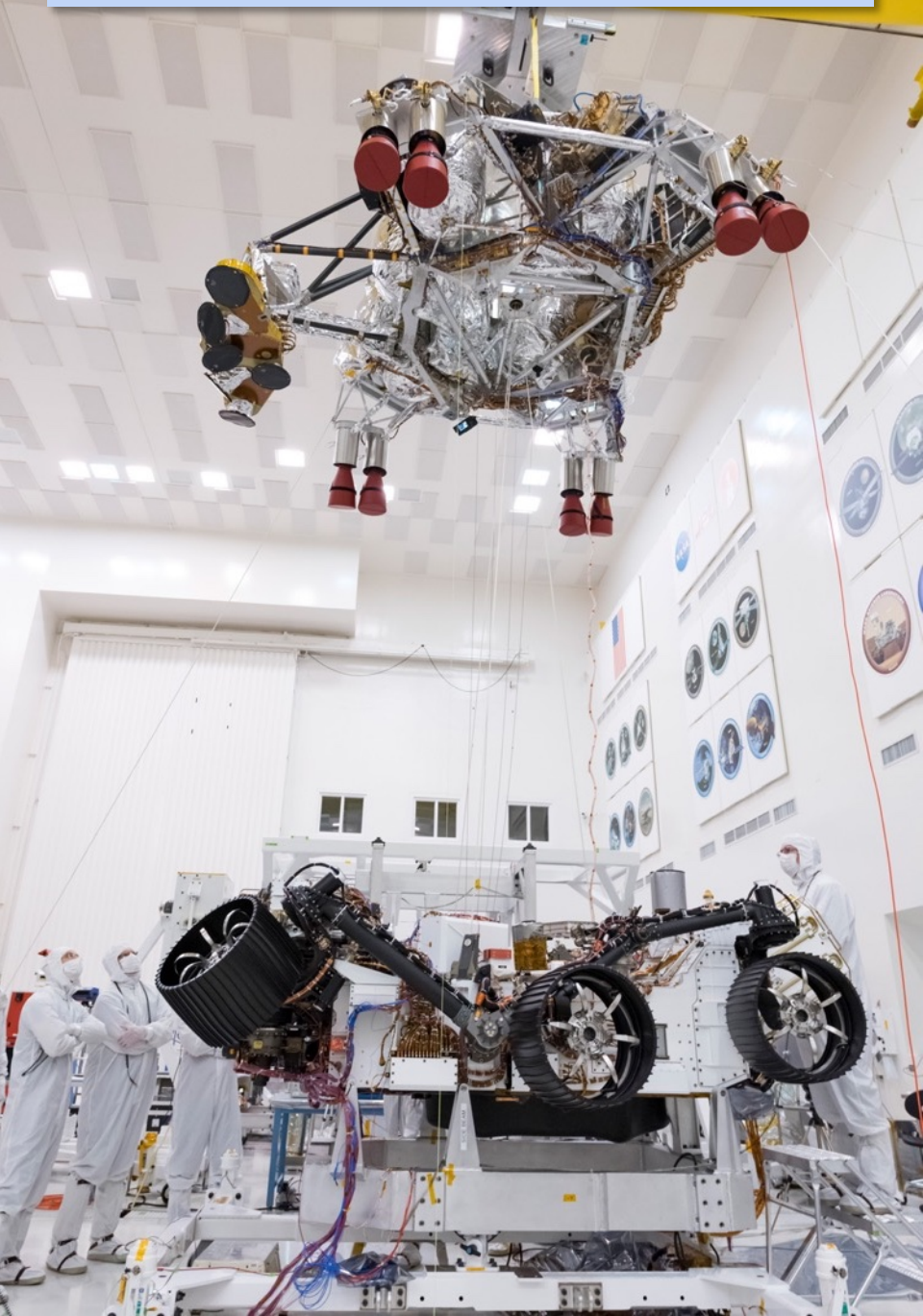
Rover and "Skycrane" Separation Test
