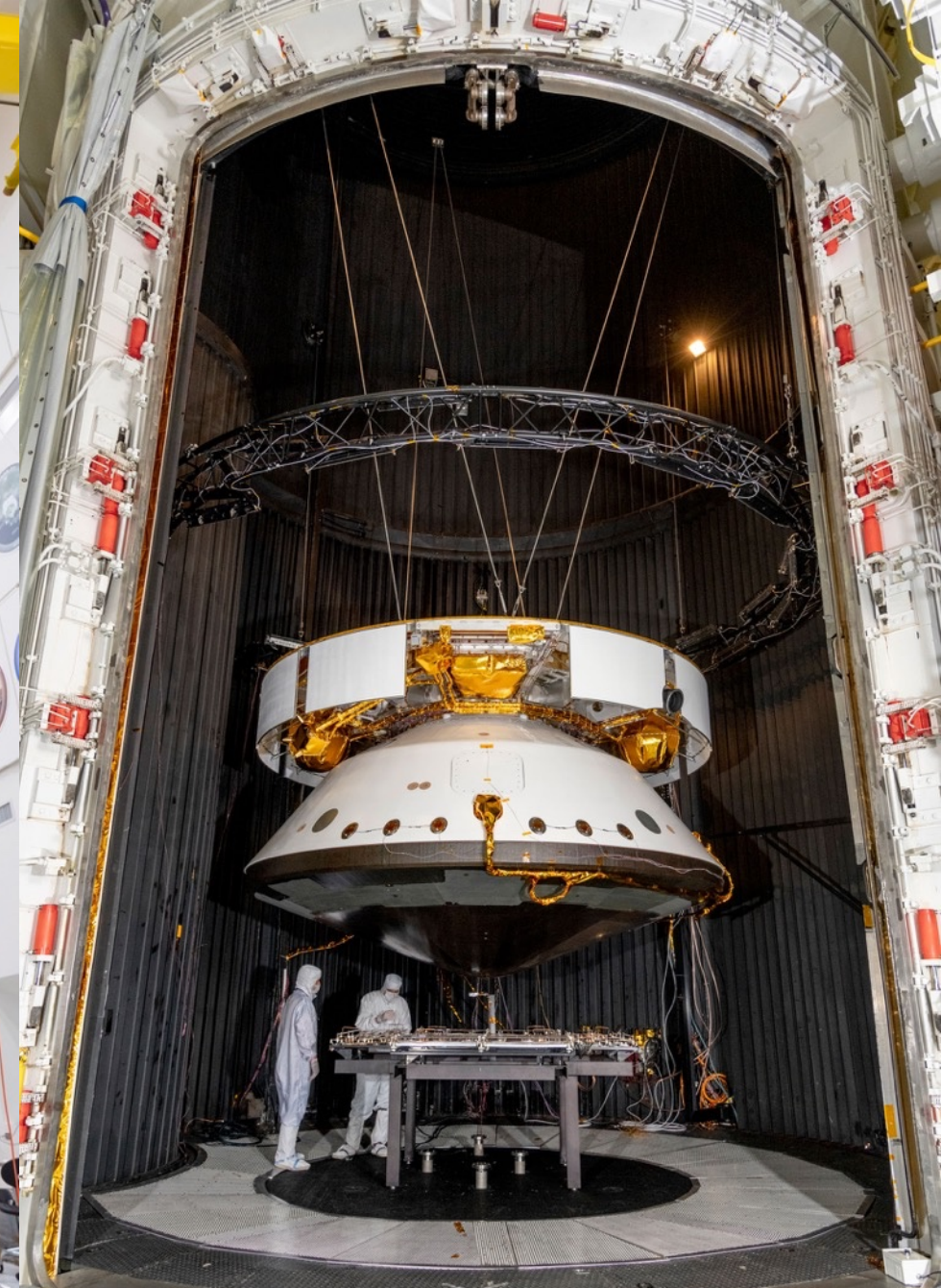
Spacecraft Thermal Vacuum Test
