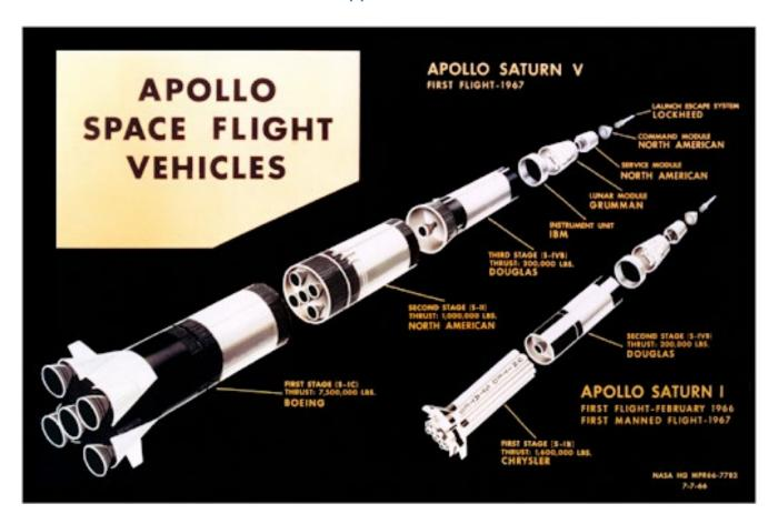
Almost every rocket has multiple "stages". A stage, in general, is a portion of the rocket that can be separated while still allowing the rest of the rocket to function correctly. For the Saturn V, there were three stages. During liftoff, only the bottom most stage fired its engines. Then once the first stage was empty of fuel, it was released by the rest of the rocket and the second stage would ignite its engines to continue the journey.
