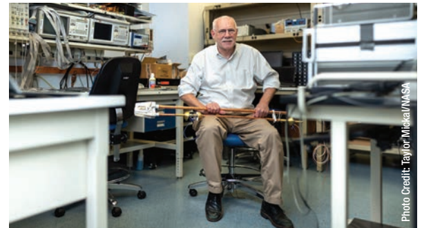
Dynamo-II Principal Investigator Rob Pfaff is holding a unique boom system developed at Goddard. Its dual sensors will measure AC and DC electric fields as part of the Dynamo-II sounding rocket mission in 2020.
