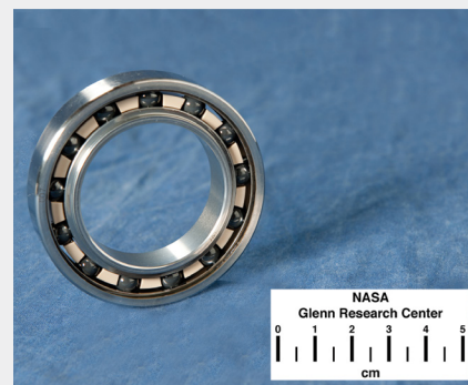
FIGURE 2: NiTi alloy ball bearing provides for shock tolerant, corrosion immune operational capability for the most demanding bearing applications.
