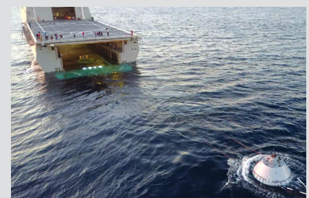
Aerial view of the USS Anchorage as the CM mock-up is recovered into the well deck during URT-7. The image was extracted from video recorded by Jamie Peer of NASA.
