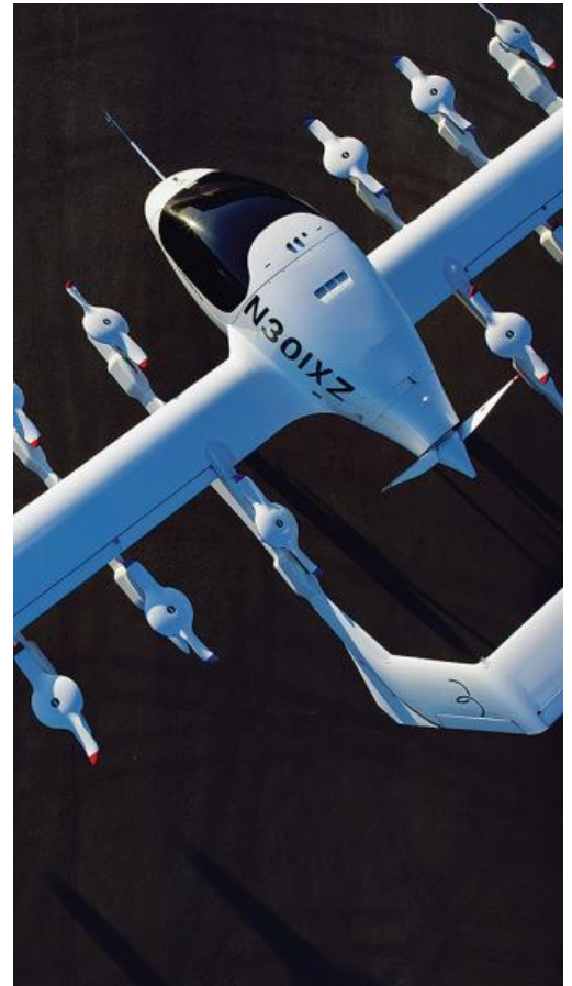
Kitty Hawk's autonomous Cora is in advanced stages of flight testing in California and New Zealand. Credit: Cora
