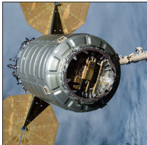
SEOPS, LLC SlingShot Dispenser mounted on the Cygnus Spacecraft. Credit: NASA/Northwest Nazarene University
