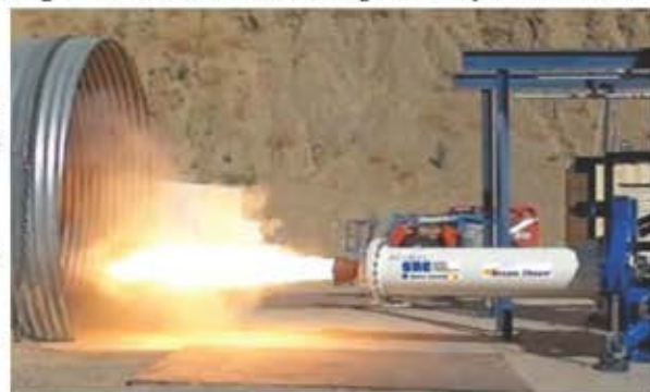
Figure 1-2. Hybrid Rocket Motor Test. Provides safe, non-toxic propulsion system for aborts, orbit adjust, and deorbit.
