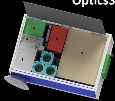
1 VACCO 3-nozzle cold gas thruster; 2 SWIFT SLX radio; 3 Batteries; 4 Avionics bus/shielding; 5 NISTEx-II interferometric star tracker; 6 X-ray camera assembly; 7 Instrument electronics/shielding; 8 VACCO cold gas generator; 9 X-ray camera/star tracker viewing ports.
