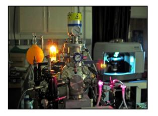
The NASA Ames **ICEE** (Institute for Carbon Evolution Experiments) Facility is a state-ofthe-art facility comprised of a high-vacuum (HV) chamber with in-situ capabilities and an external Raman microscope system.
