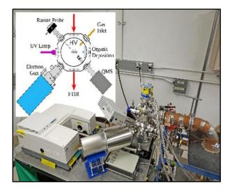
ICEE facility setup showing the internal schematics of the HV chamber, the locations of the 100 keV electron gun, UV light source and mass spectrometer attached as well as the in-situ capabilities.
