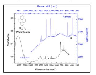
Raman (blue) and IR (black) spectra of a water matrix-isolated PAH molecule (pyrene) sample collected via in-situ Raman and IR.
