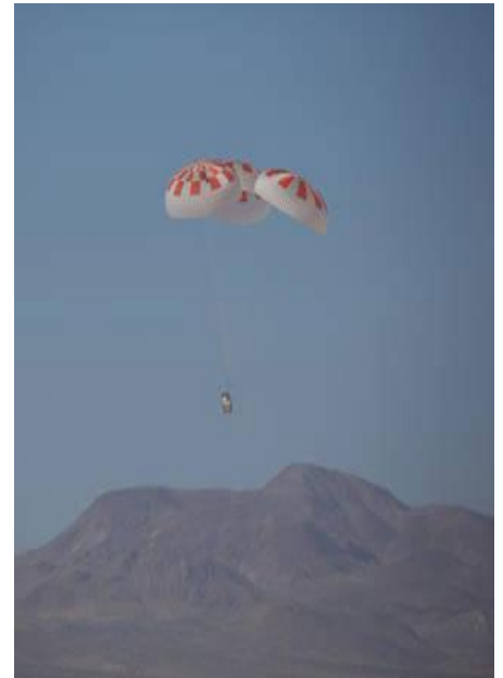
SpaceX performed its fourteenth overall parachute test supporting Crew Dragon Development March 4, 2018, over the Mojave Desert in Southern California. The test demonstrated an off-nominal, or abnormal, situation, deploying only one of the two drogue chutes and intentionally skipping a deployment stage on one of the four main parachutes. Photo credit: SpaceX
