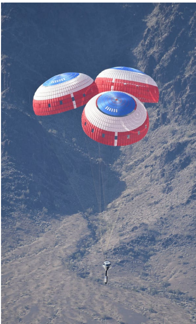
Boeing conducted the first in a series of reliability tests of its CST-100 Starliner flight drogue and main parachute system Feb. 22, 2018, over Yuma, Arizona. Photo credit: NASA
