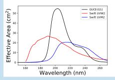
The high-efficiency delta-doped CCDs and hightransmission anti-reflection coatings enable GUCI to achieve a larger effective area than *Swift*-UVOT, despite a much smaller aperture (13 vs 30 cm)
