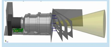
13 cm, 6 element refractive telescopes • High-efficiency delta-doped CCD detectors (JPL) • High-transmission GdF<sub>3</sub> anti-reflection coatings (GSFC) • Deployable straylight baffles
