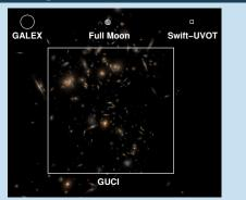
With a 50 deg<sup>2</sup> field-of-view, GUCI will rapidly (< 2 hours) image gravitational wave localizations to characterize the prompt UV signal from binary neutron star mergers.
