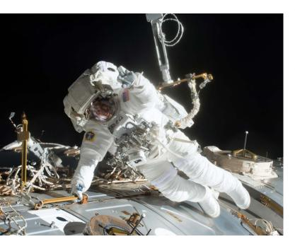
Spacesuits have multiple layers to support life and protect astronauts. The first two internal layers make up the liquid cooling and ventilation garment. These layers are made up of spandex fabric and plastic tubing. The next layer is a pressure bladder made of urethane-coated nylon followed by a pressure-restraining fabric layer. This is followed by seven layers of a thermal micrometeoroid garment. All of these specialized layers come together to form the spacesuit.
