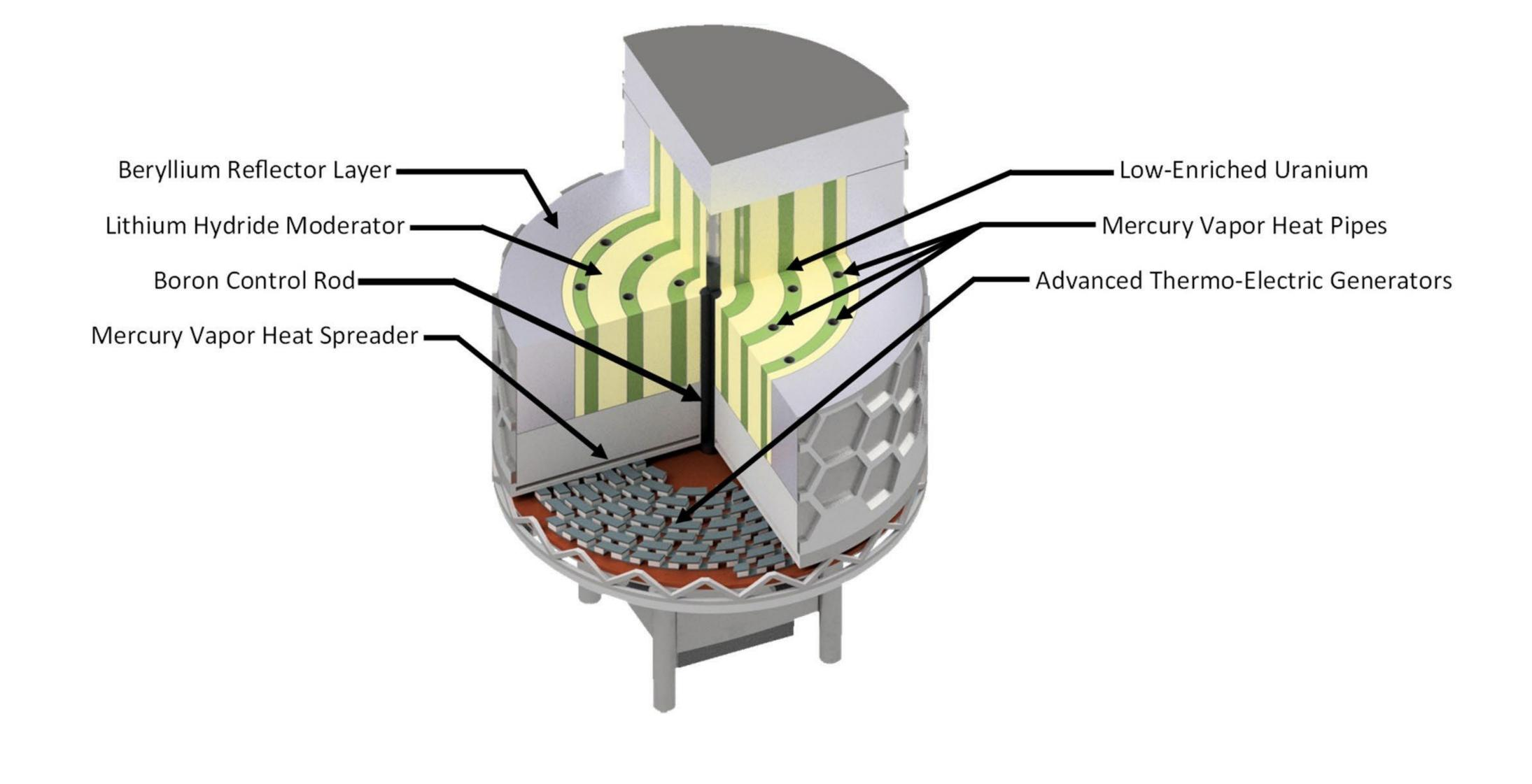
Nano-reactor remains inactive until parking orbit has been reached
