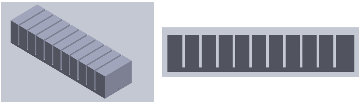
Figure 9: Knee soft-robotic actuator prototype #1 with integrated strain-limiting layer: isometric view (left) and front view (right). The chambers are connected internally through the strain-limiting layer.
