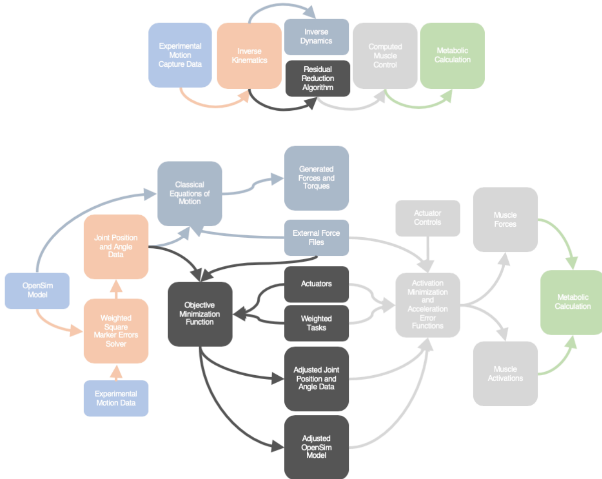
Figure 4: The overall computational procedure using OpenSim is summarized above. Experimental Motion Capture data relates to the experimental data collected from tests or studies (we used already existing walking data available in OpenSim). Inverse Kinematics computes the joint angles and positions of the human model based on the experimental motion capture data. Inverse Dynamics solves for the forces and torques of the different bodies and joints in the human model. The Residual Reduction Algorithm slightly adjusts the center of mass of the model and associated kinematics to improve dynamic consistency. The CMC tool computes a set of muscle activations and forces that drives the dynamic model to track the desired kinematics. Finally, muscle and actuator activation data are then used by the Metabolic Calculator to find the total energy expenditure for the specific motion being analyzed.
