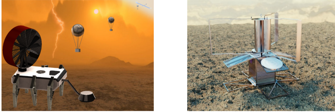
Fig. 1. Recent examples of Venus surface mission concepts, currently baselined using wind power generation including an Automaton Rover (left) and the LLISSE Lander (right). These landers could be powered using power beaming approaches, to address the inherent uncertainties and limits imposed by sporadic/low velocity Venus surface winds.
