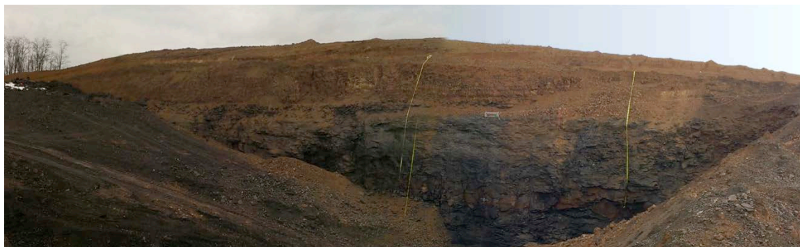
Figure 155: Robotic exploration and modeling tests in a mine pit. Yellow streamers mark the edges of the portion of the mine’s high wall that was the focus of modeling for this experiment.
