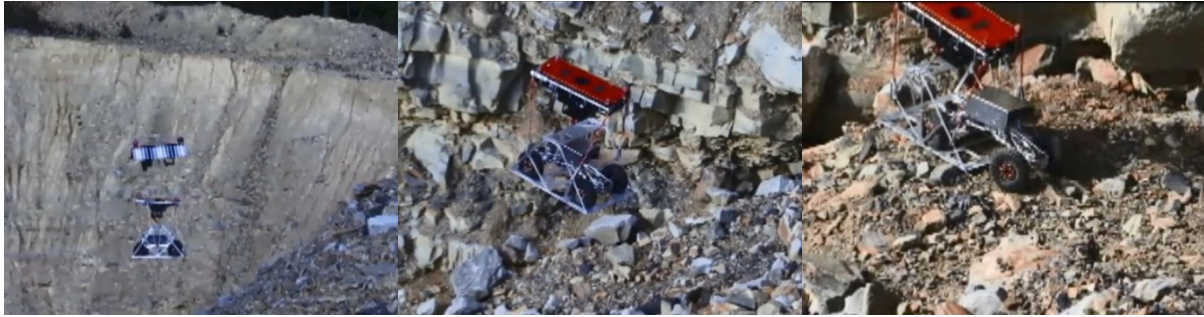
Figure 77: Deployment of Krawler into pit by Tyrobot
