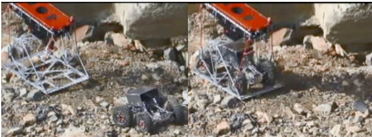
Figure 79: Krawler approaches and re-docks with Tyrobot, facilitating re-charge or transport to another location in the pit.
