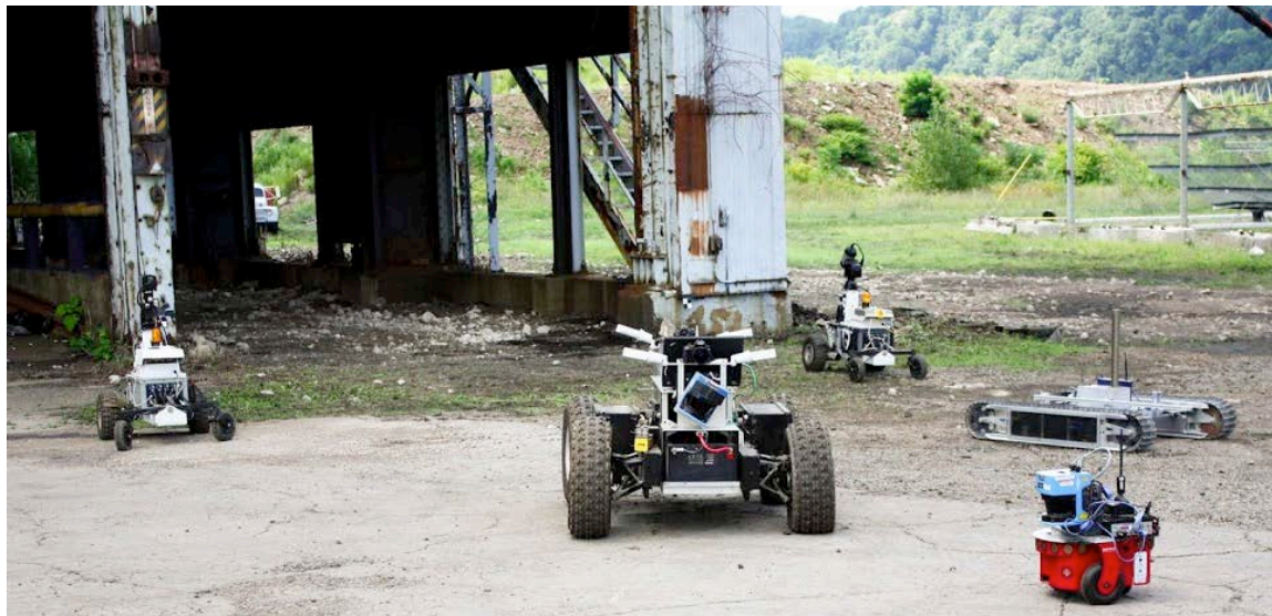
Figure 154: Multi-robot team in front of a building used to construct an analog tunnel and conduct experiments in multi-robot cave exploration for the NASA STTR Multi-Robot Systems for Subsurface Planetary Exploration
