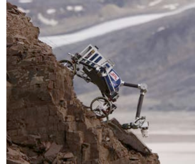
Figure 17: Cliff-bot utilizes two robots as anchors with tethers to assist in the motion of a rappelling robot. [37,38]
