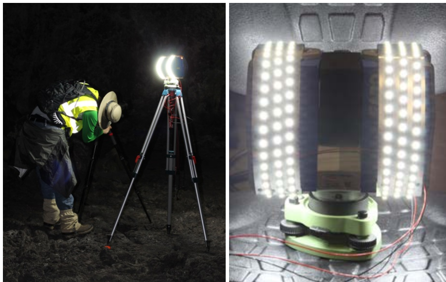
Figure 111: Experimental setup for lava tube wall modeling. An intern adjusts a camera next to the LIDAR scanner in Indian Tunnel (left). The banded LED illumination provides a wide, diffuse area of illumination. Lateral symmetry reduces harsh cast shadows (right).
