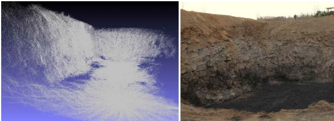
Figure 85: A “dewarped” geometric point cloud of mine test site (left) and an image of the same scene (right).
