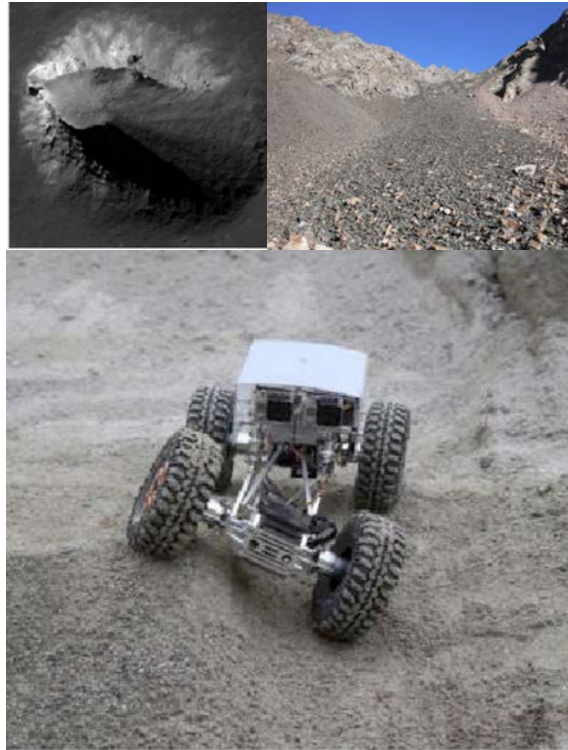
Figure 26: Lunar pit with a scree slope (top left), terrestrial scree slope (top right), and scree slope descender prototype (right).
