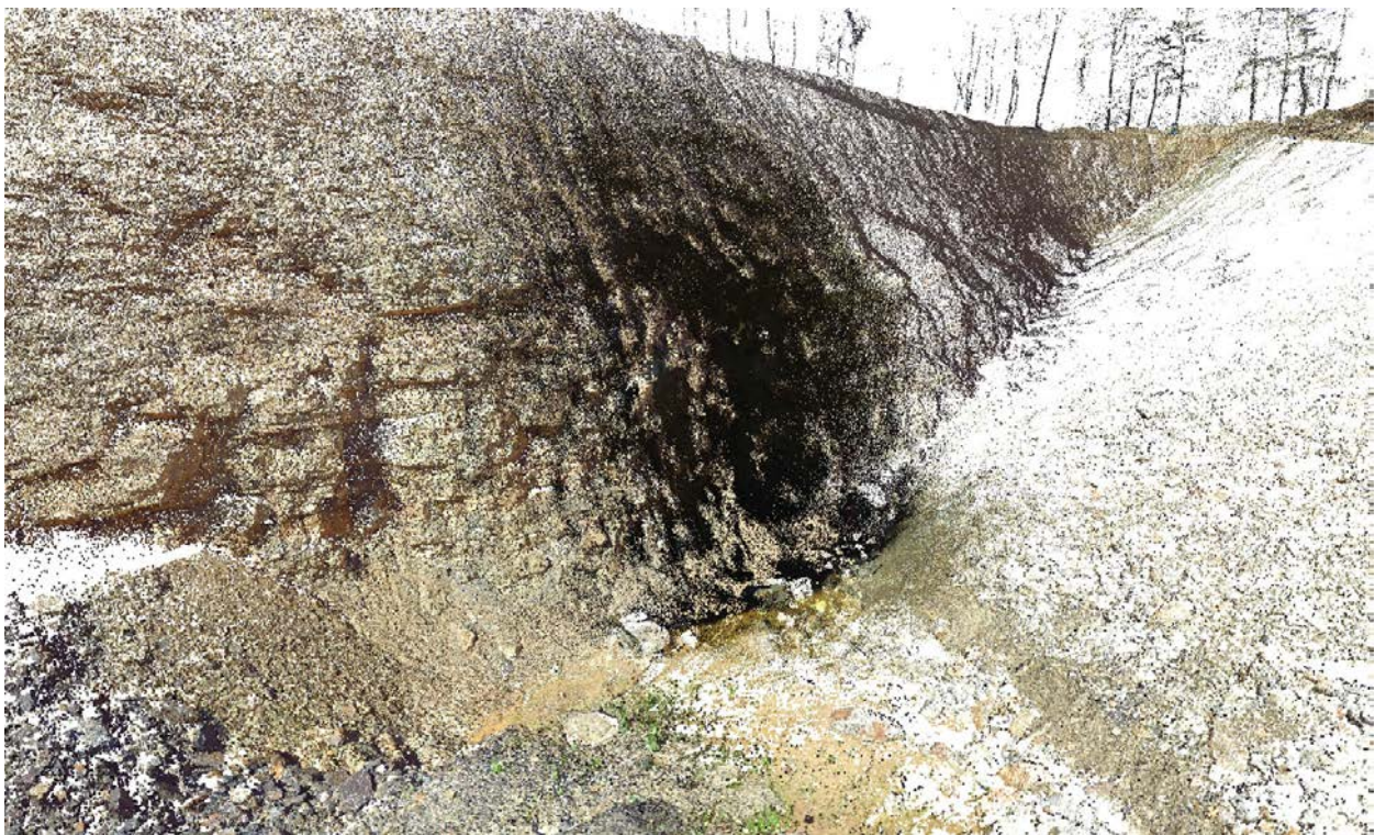
Figure 93: Third of four robot scans (saturated section) overlaid with FARO ground truth measurements
