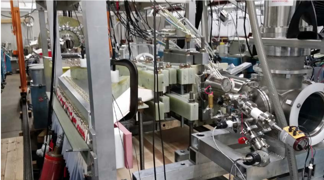
Figure 27. Feedplate clamping on current FRC liner source experiments at PDL.
