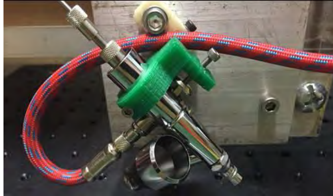
Figure: Computer controlled polymer spray nozzle mounted on precision computer motion controlled 2 axis gantry
