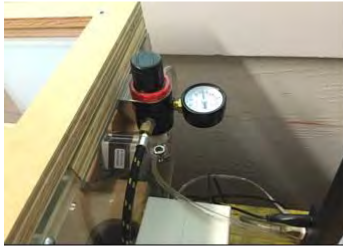
Figure: Spray pressure is regulated and adjustable
