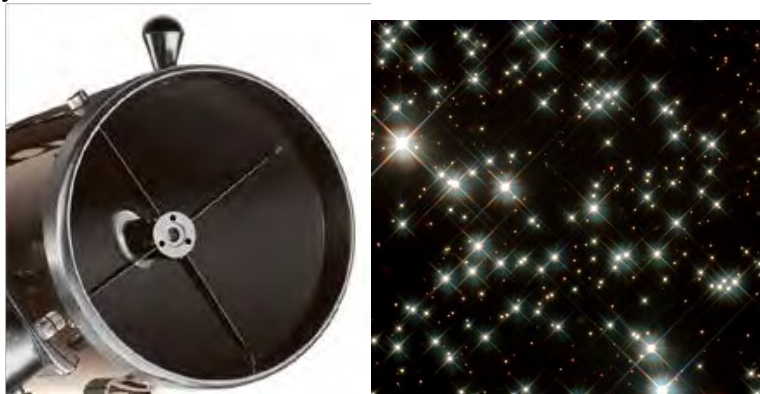
Figure: A spider support holding a secondary mirror and the resulting spider diffraction.
