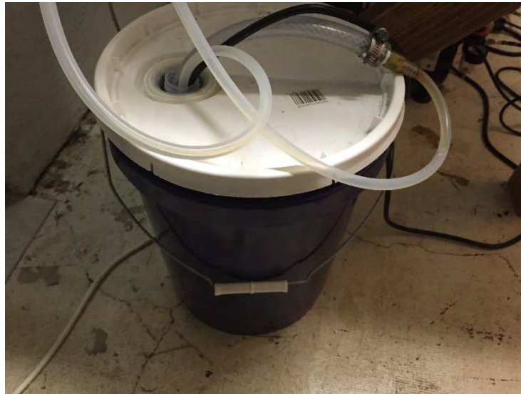
Figure: Low tech CO 2 laser cooling system
