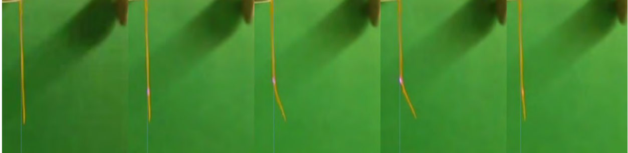
Figure: Note in the final frame a relaxation resulting in return to near vertical displacement. Also note this is not simply melting as working being performed against gravity by this optical machine.
