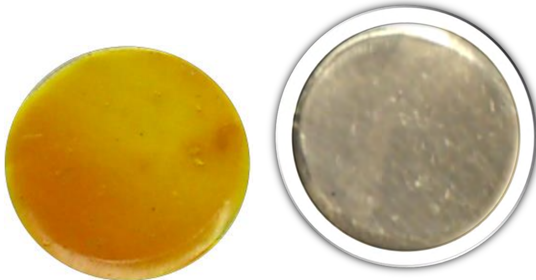
Figure: formed polymerized round OCCAM OSSAPOS PM Star AzoPoss membrane and a crude mold.
