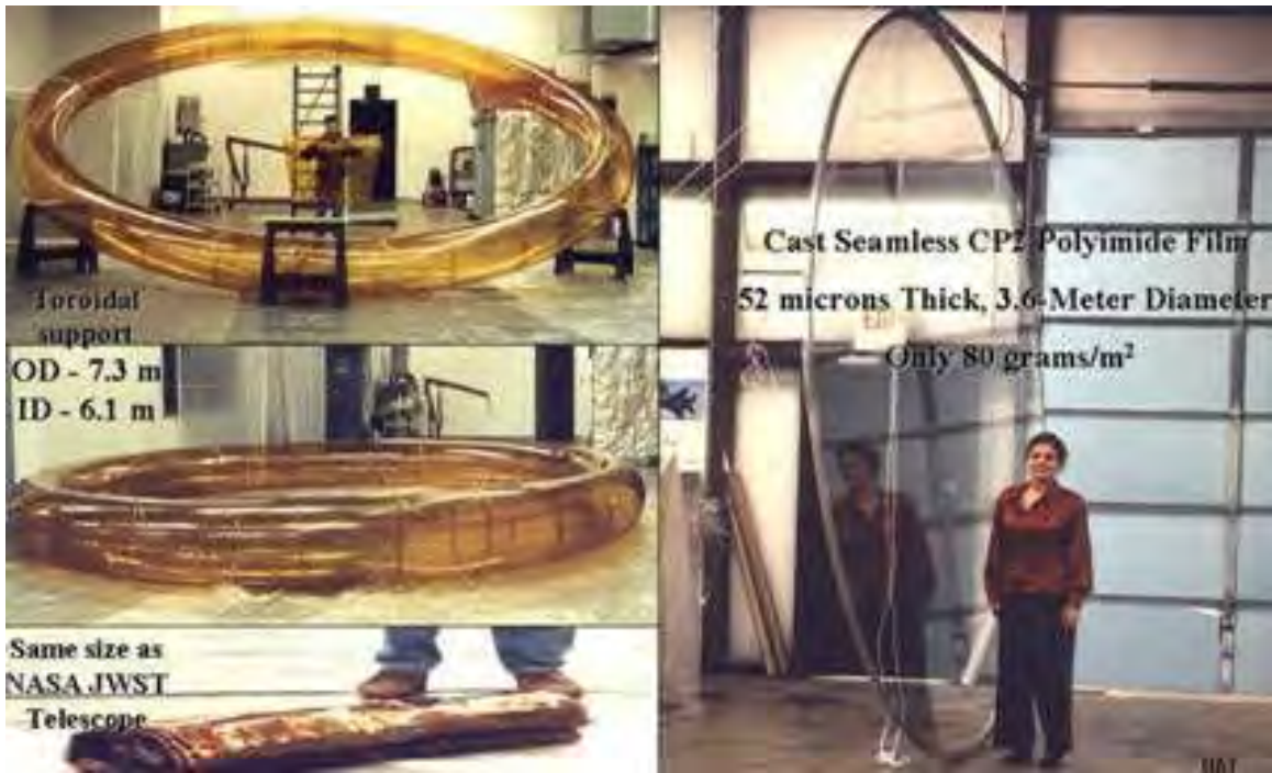
Figure: Existing toroidal mirror support JWST size (From Colleagues at UAT Huntsville)
