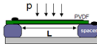
Figure 24 Piezoelectric sensor construction (image credit: Xerox PARC)
