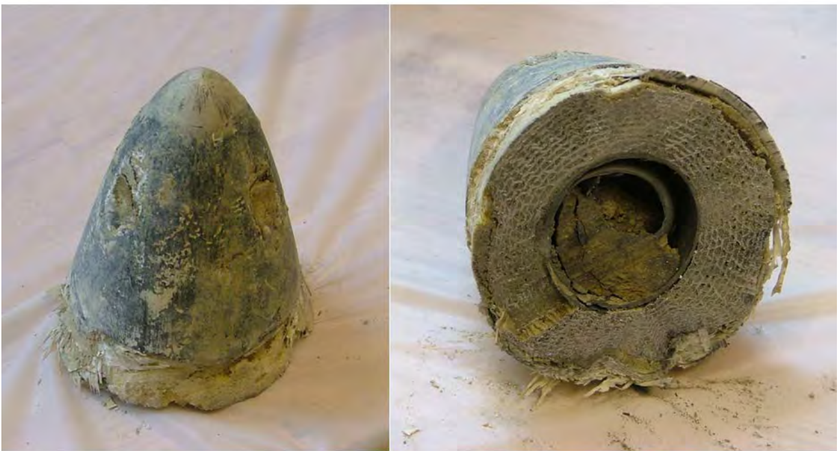
Figure 19. Top and rear views of the nose cone from the supersonic flight. Playa is seen to fill the sample ports and this material is seen in the interior sample collection region.
