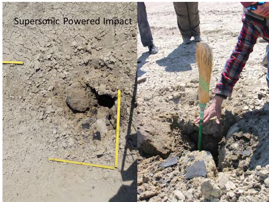
Figure 17. Impact crater for the powered supersonic flight. The site shows the impact of the fin and body tube though there was no sign of the rocket itself.
