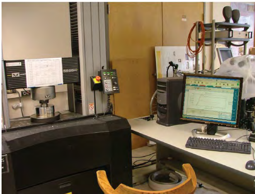
Figure 7. Compressional test stand (left hand side) and control computer (right hand side).
