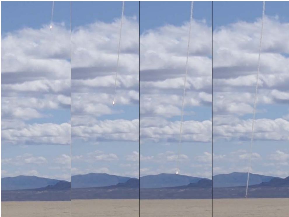
Figure 15. Impact of the penetrator at an estimated speed of Mach 1.4.
