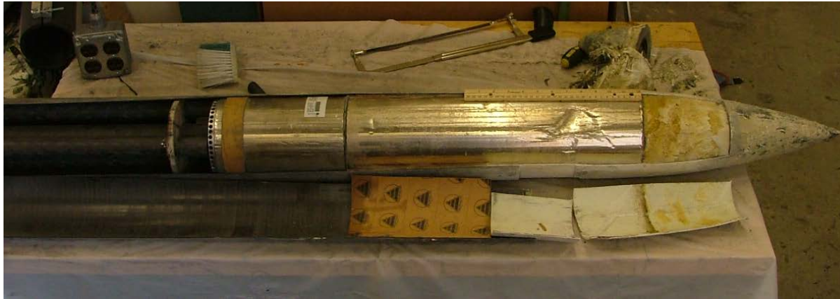
Figure 13. View of the internal components of the penetrator after impact. It is seen that beyond some denting of the part of the crumple zone the internal components are essentially intact.
