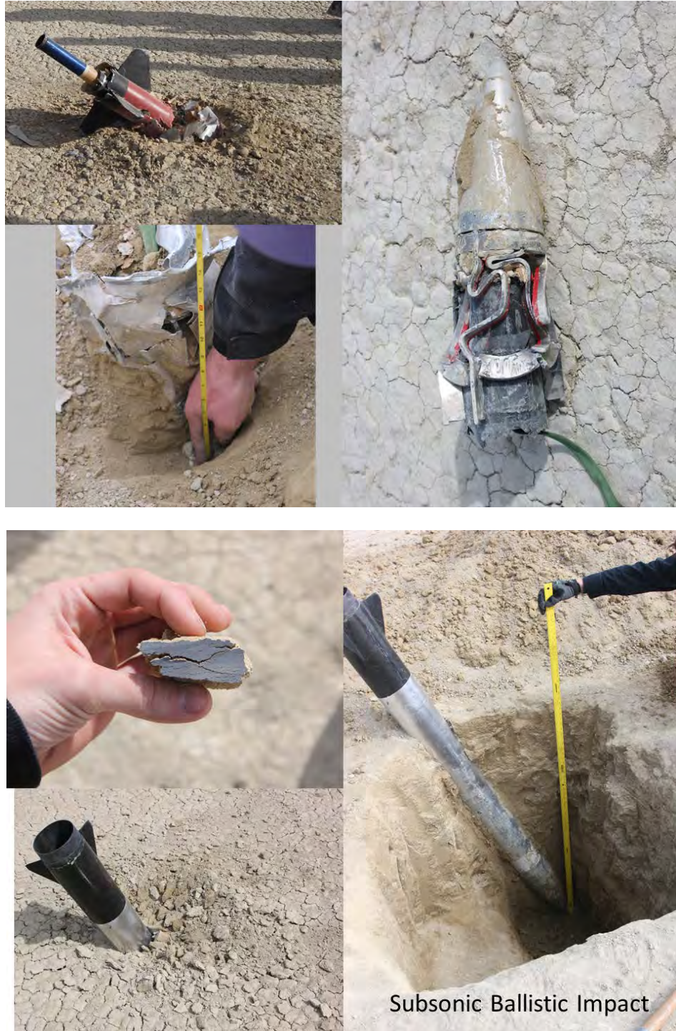
Figure 12. Comparison between impacts from 2012 (top) showing major structural failure with penetration to 22in and the NIAC 2013 test (bottom) where the rocket penetrates to 4ft with a larger impact crater, stress fractures in the playa and minimal damage to the rocket.
