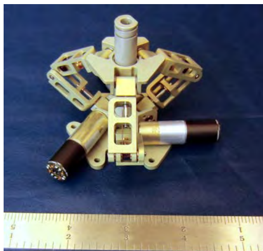
Figure 37. COBRA™ Gimbal Developed for CubeSat Applications. The COBRA gimbal is a Canfield-joint carpal-wrist mechanism that provides azimuth, elevation, and plunge motions over a full hemispherical work space.
