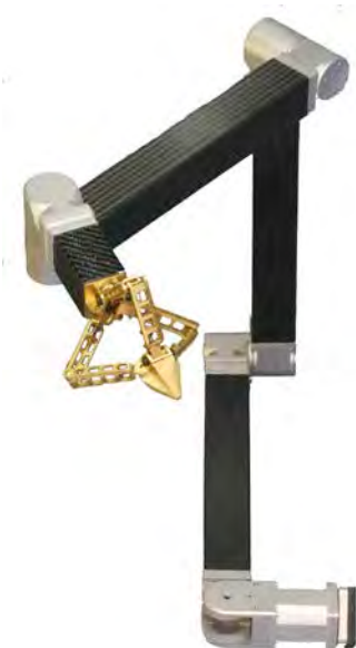
Figure 36. KRAKEN Robotic Arm. The KRAKEN is a 7DOF robotic arm with 1-m reach. Two KRAKEN arms will stow within a 3U CubeSat volume.
