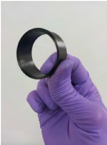
Figure 32. Roll of Carbon-Fiber/PEEK composite tape. CF/PEEK unidirectional prepreg tape can be wound compactly, yet has sufficient stiffness to be fed into a forming mechanism.
