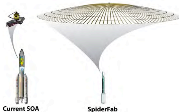
Figure 1. SpiderFab Value Proposition. On-orbit fabrication of spacecraft components enables higher gain, sensitivity, power, and bandwidth at lower life-cycle cost
