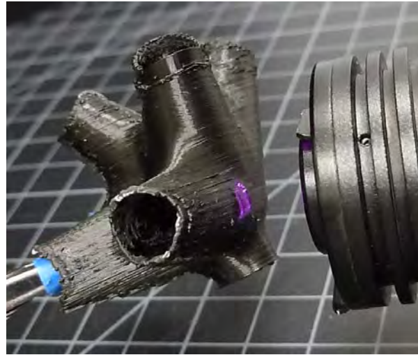
Figure 46. Testing of Plastic Joint Surface Pre-Heating with 700mw IR Laser. We have experimented with non-contact methods of heating the joint material to bring cold parts into the processable range.
