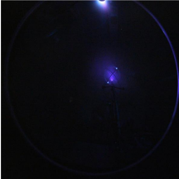
Figure 36. Magnetoshell operating with internal gas feed and intercepting only MPD plasma. Shown is 50 sccm internal feed, 3 Joule RF, and 1 ms MPD discharge at 1.2 kV and 1 ms delay.#20165
