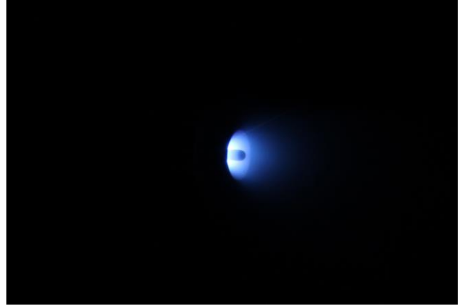
Figure 29. Pulsed MPD operating with an argon propellant and 2 ms discharge.
