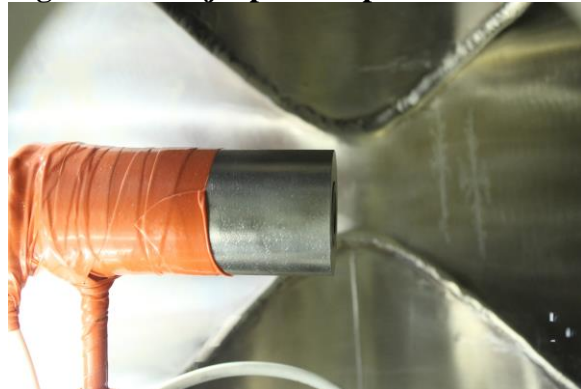
Figure 27. Arcjet mounted in the 'Junior' test facility.
