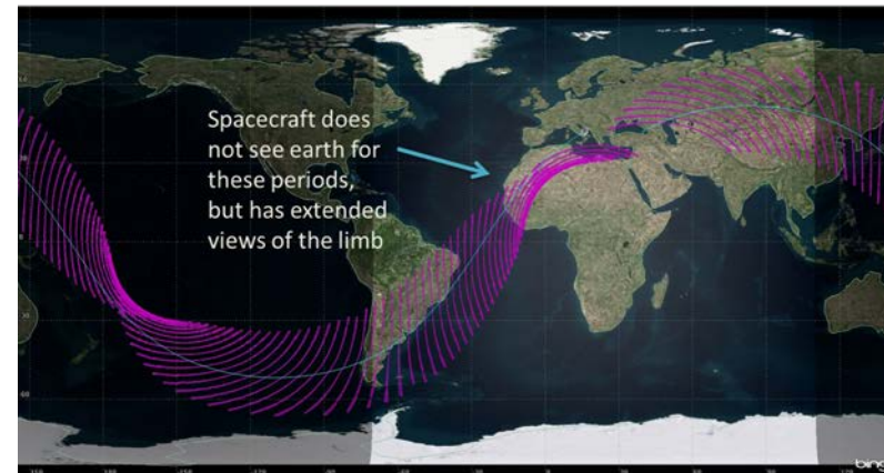
Radiometer Ground Track on Equinox
