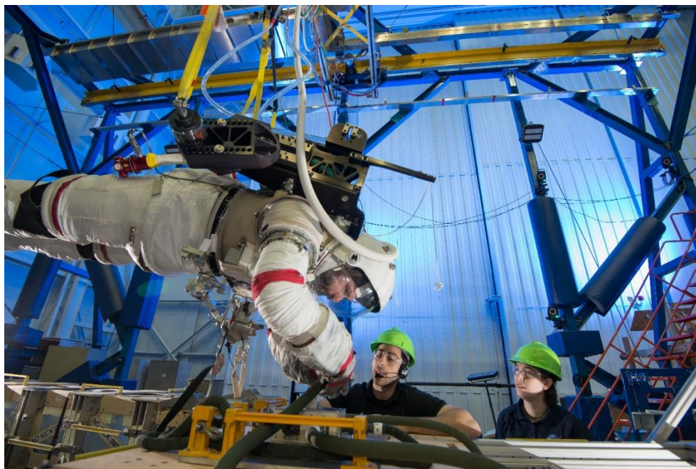
Figure 3. Suited subject in the EMU performs quick disconnect task board as part of the EVA Human Health and Performance Benchmarking Study.
