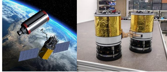
Figure 1 – (Left) Application to free-flying robotic spacecraft grasping and manipulating partially uncharacterized non-cooperative objects, (Right) Stanford Spacecraft Robotics Facility, one of the test beds that will be used in this investigation.
