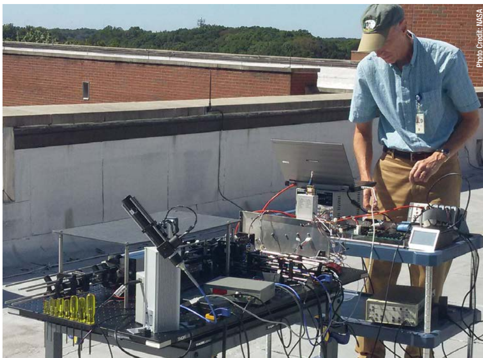
Steve Bailey helped physical chemist Tom Hanisco develop a portable instrument to measure hydroxyl, a chemical that cleanses the atmosphere of highly damaging methane. With this instrument, Hanisco obtained initial measurements from a rooftop at the Goddard Greenbelt campus.
