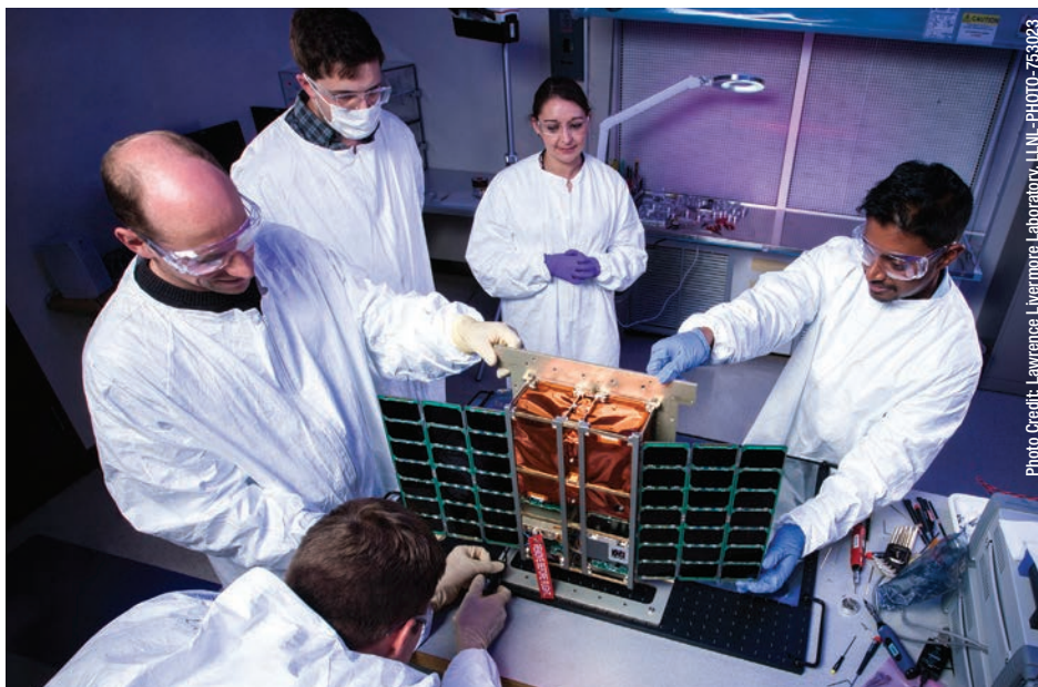
Technologists integrate a Goddard-developed instrument into Lawrence Livermore National Laboratory's (LLNL) CubeSat bus. Those pictured include LLNL's Lance Simms (front) and from left to right: Vincent Riot (LLNL), A.J. DiGregorio (Goddard), Jennifer Young (Goddard), and Guru Ramu (Goddard).
