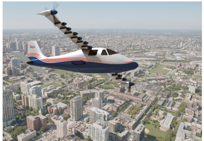
Figure 1. This artist's concept of NASA's X-57 Maxwell aircraft shows the plane's specially designed wing and 14 electric motors. Credit: NASA Graphic / NASA Langley / Advanced Concepts Lab, AMA, Inc.
