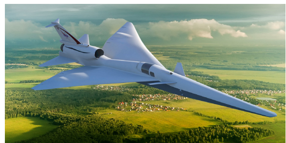
Figure 7. NASA’s newest X-plane, the X-59 QueSST, will fly over communities to measure sound levels and how people react to quieter sonic thumps.
