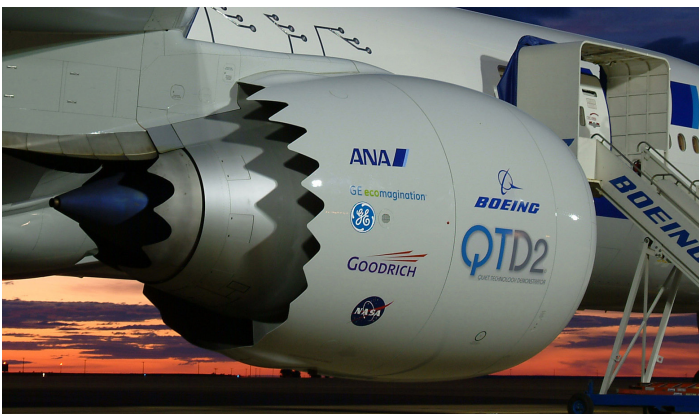
Figure C. Final chevron shapes—asymmetrical—in place on engine casing and nozzle.
