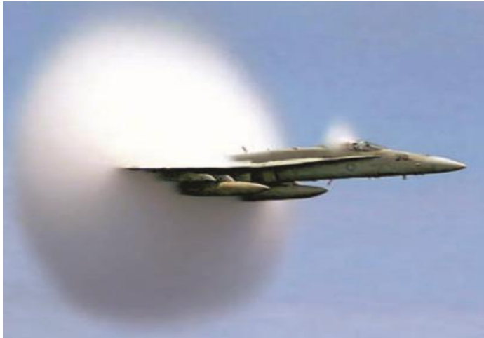
Jet breaking the sound barrier showing condensation of air shock wave
