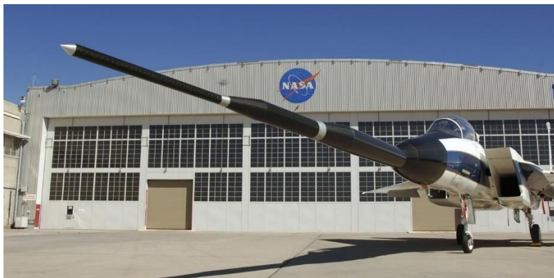
NASA's F-15B testbed aircraft with Gulfstream Quiet Spike sonic boom mitigator is a precursor to the X-59
