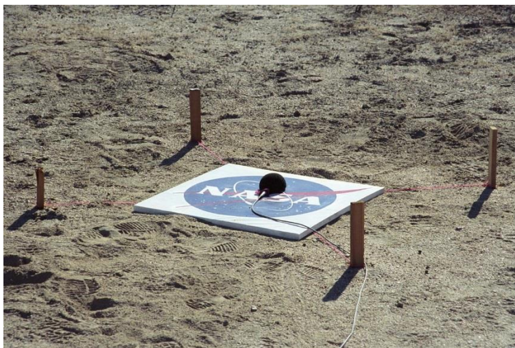
One of many microphones to record sonic booms from the F-5E SSBE aircraft
