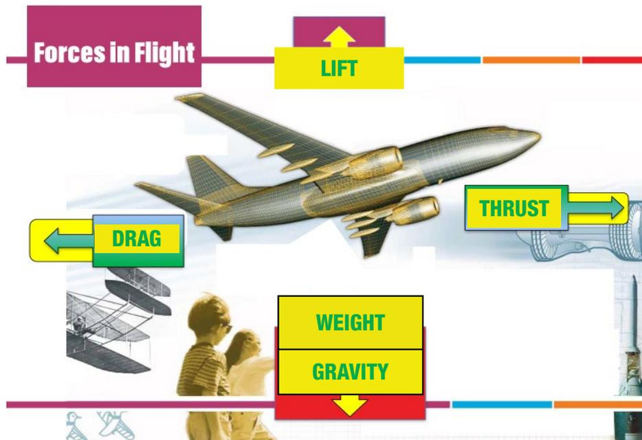
There are four forces in flight that enable an airplane to fly: Thrust, Drag, Weight, and Lift.
