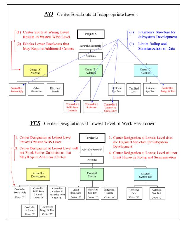
Figure 3-17: Center Breakout Guidance for a WBS
