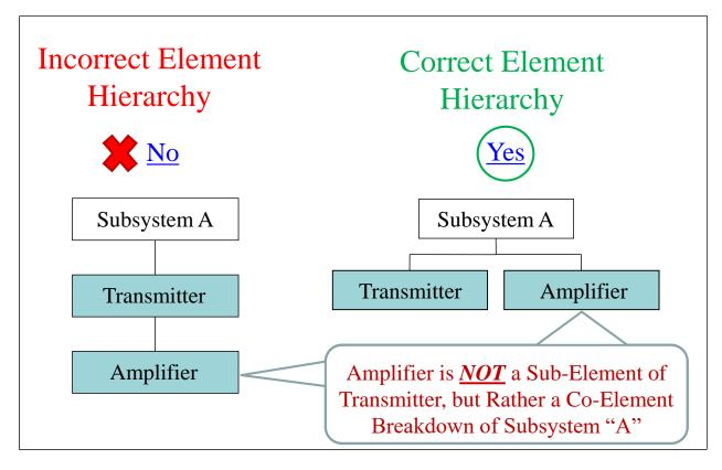
Figure 3-18: Illustration of Incorrect Element Hierarchy
