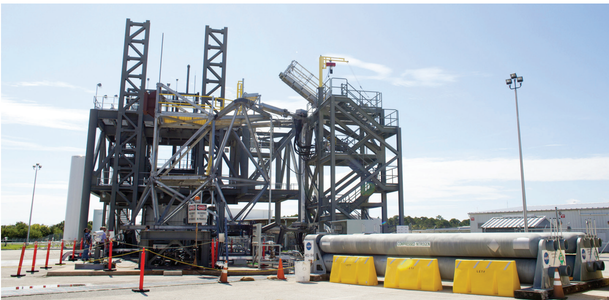
The vehicle motion simulator, or VMS, which simulates all of the movements a space vehicle could experience from rollout to launch at NASA's Kennedy Space Center in Florida. Testing of umbilical's are ongoing in support of the agency's Space Launch System rocket and Orion capsule. Photo credit: NASA
