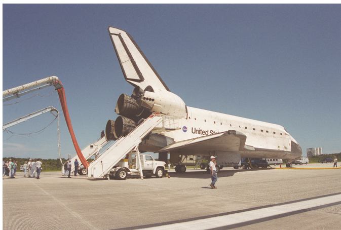
Umbilicals are attached to purge the vehicle of any possible residual explosive or toxic fumes.
