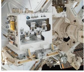
The Robotic Refueling Mission, or RRM, module was temporarily installed on the Dextre robot's Enhanced ORU Temporary Platform on the International Space Station. RRM resided there for nearly two months before being transferred to its permanent location on an external platform fit for its robotic demonstrations.
