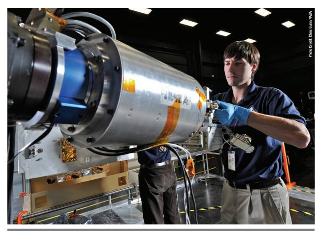
Geared up and ready to go, SSPD team member and robot operator Alex Janas attaches a Robotic Refueling Mission, or RRM, tool onto the industrial robot arm before simulating an RRM servicing task.
