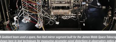
A Goddard team used a spare, five-foot mirror segment built for the James Webb Space Telescope shown here to test techniques for measuring picometer-sized distortions in observatory optics and support structure.
