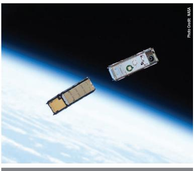
The bread loaf-sized lceCube was deployed from the International Space Station in May. One month later, it began science operations gathering global data about atmospheric ice <u>clouds in the submillimeter wavelengths.</u>
