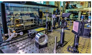
The MARLI instrument breadboard is encased inside the clear case in the background. The cylindrical object in the foreground with the silver-colored outer shell is the optical etalon used in the lidar receiver.
