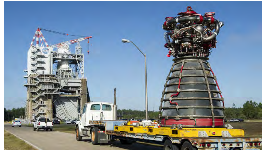
Transporting an RS-25 Engine
