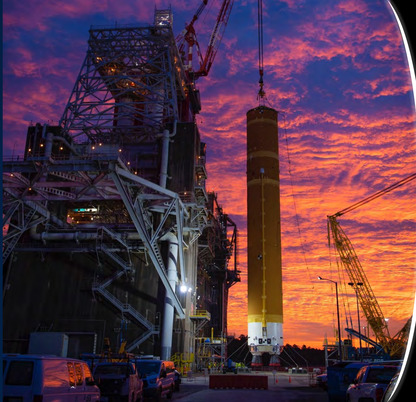
Space Launch System Core Stage being lifted into the B2 Test Stand on January 21-22, 2020
